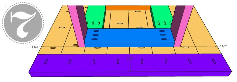
Now, center the table base on the bottom of the table top. Secure the base to the top with 2 1/2" wood screws. Do not use wood glue here.
