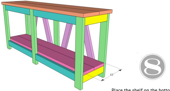
Place the shelf on the bottom aprons, and attach them using wood glue and 2.5" pocket hole screws. It helps to lay the table on it's back or side to attach these boards.
