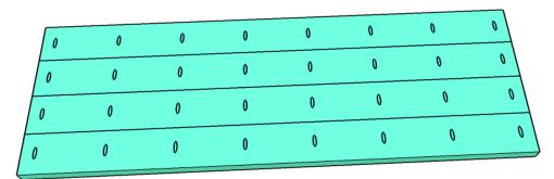
Cut the short planks, drill 1 1/2" pocket holes and attach them to the table legs with 2 1/2" pocket hole screws.
