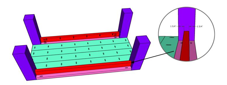
Cut the short apron pieces to fit, drill 1 1/2" pocket holes and attach them to the legs and long planks with 2 1/2" pocket hole screws.
