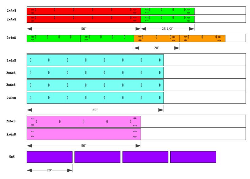
Cut the long planks, drill 1 1/2" pocket holes and attach them together with 2 1/2" pocket hole screws.
