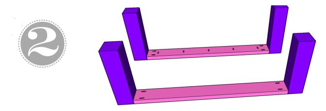
Now, attach the legs and short planks to the long planks with 1 1/2" pocket hole screws.
