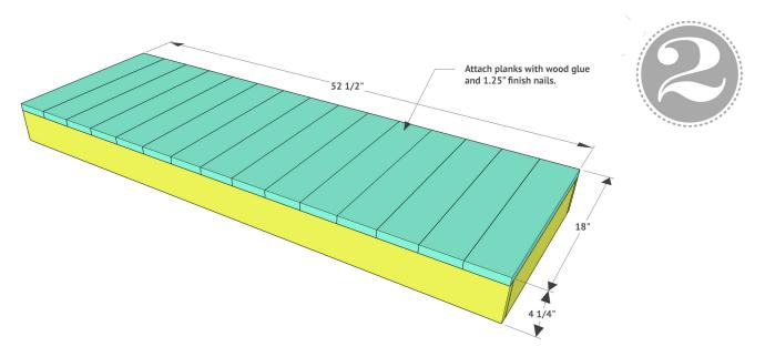
Next, line up 15 planks along the top of both frames and attach them using wood glue and 1.25" nails.
