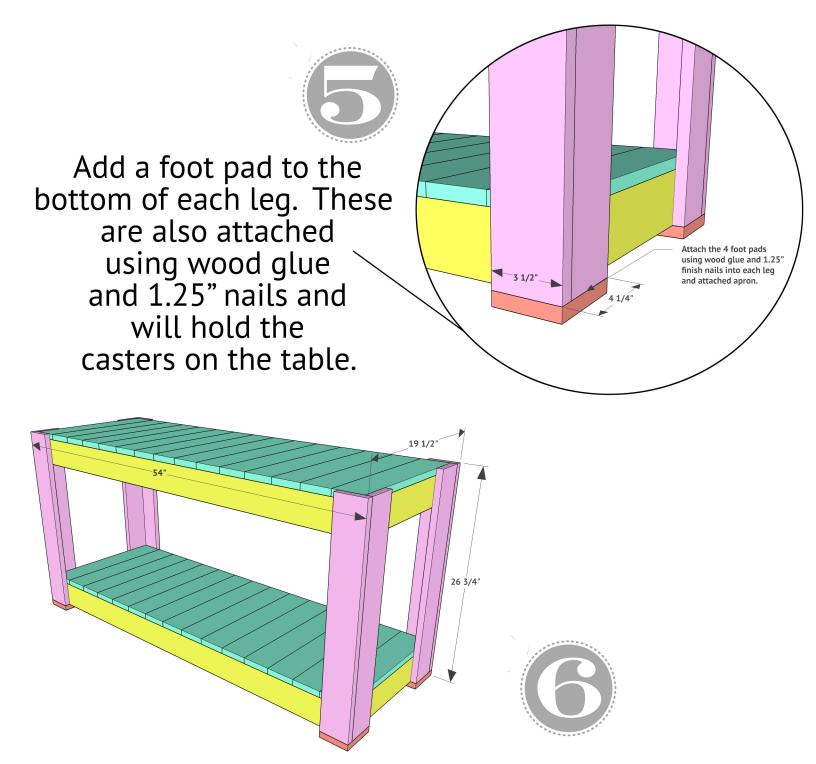
Final step is flipping the console over and attaching the casters. These will attacht to each foot pad using wood screws. Once they are attached, flip it back over and stain or paint your table to fit your style. Be sure to tag us in your finished projects! We love seeing and sharing them!
