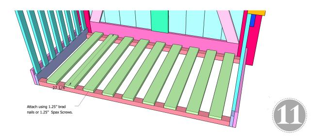
Attach the rails to the cleats using either 1.25" finish nails or 1.25" Spax screws. Now drop in the mattress and you're ready to go!
