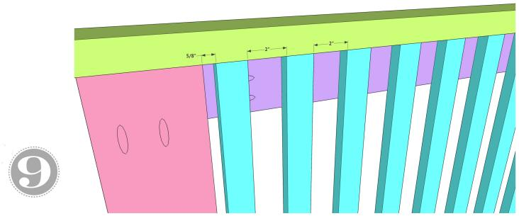
Attach the crib rails just like you did the side rails. These are also placed every 2" and attached with wood glue and finish nails. See how they cover the pocket holes!
