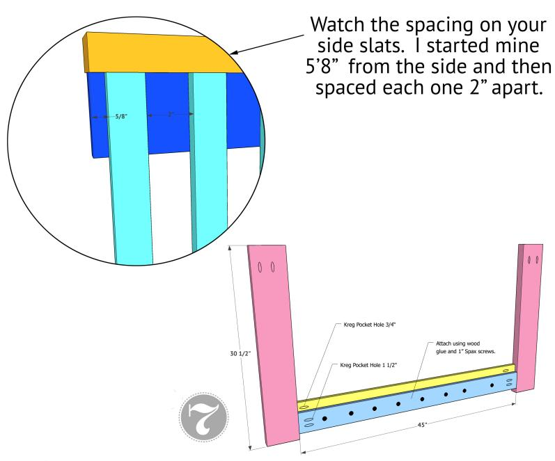
Time to start on the front of the crib. First, attach the two bottom boards using wood glue and 1" Spax screws.
