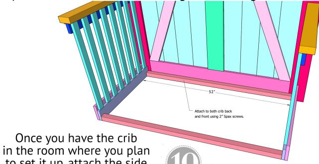
in the room where you plan to set it up, attach the side pieces to the back by using 2.5" pocket hole screws through the sides and into the back. You can also add some 2.5" Spax screws through the back and into each side rail if you want to.
