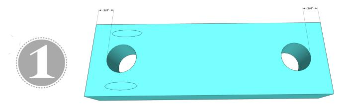
After making all of your cuts, drill two, 1 1/2" pocket holes on one end of the top arm piece. Make sure to place the pocket holes wide enough apart so that you have room to drill the hole for your cord. Then, using a 1 3/8" forstner bit, drill a hole on each end of the top arm. I centered my holes and placed them 3/4" from each end.
