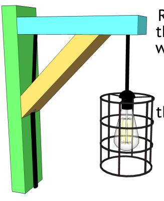
Run the cord through the holes, then attach the cross piece with wood glue and 1 1/4" brad nails. To hang, use 3" wood screws and drill from the front of the corbel into the studs behind the wall. If you don't havea stud to drill into, use wall anchors.
