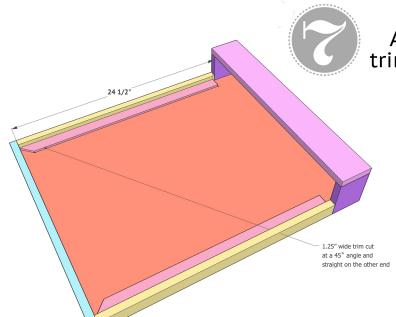
Add the decorative trim next. This trim is 1/4" thick and about 1.25" wide. There are several different styles to choose from, so go with one that you like. Attach the trim using wood glue and 5/8" nails. Notice that one end of each board is mitered at a 45° angle and the other ends are straight.
