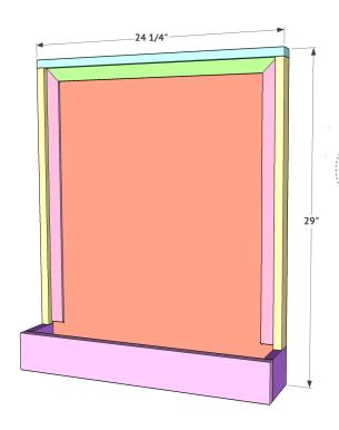
At this point you are done with assembly. Before attaching the mirror with mirror adhesive, finish the wood with paint or stain and allow it to dry. This will keep you from having to tape off the mirror and save time.
