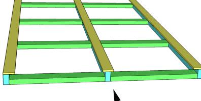
Cut the front slats, to size, and attach them to each of the three 1x2 slides with 5/8" brad nails and wood glue. The top and bottom slats should be flush with the top and bottom of the frame. The middle slat should center over the middle slide, so that there is a 3/8" overhang on each side.
