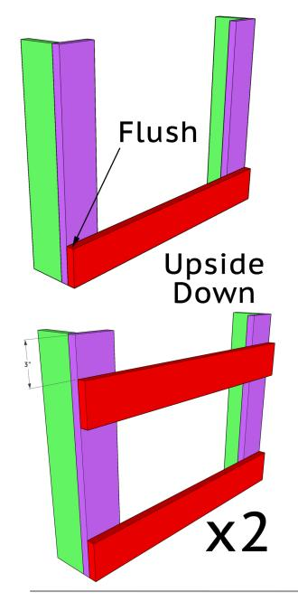
Attach a short apron piece to the edge of both legs. Make sure that the apron is attached to the side of the leg without the seam and that it is flush with the edge of the legs.
