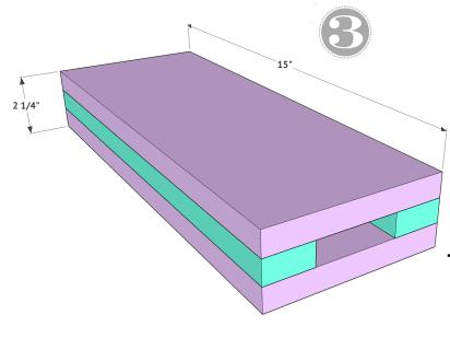
Final step is attaching the top 1x6 board. Use wood glue and 1.25" brad nails to attach it to the top of the 1x2 boards and flush.
