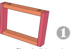
First, build two boxes for each leg assembly. These are attached using wood glue and 2.5" pocket hole screws through the horizontal boards and into the vertical boards. You want your pocket holes facing the outside of the box on this part because we will cover them with another board on the next part.
