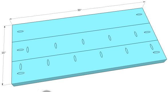
Create the shelf assmebly of the table the same way! Attach the three boards to each other using 2.5" pocket hole screws. Don't forget to add the pocket holes on each end to attach this to the leg assembly later.
