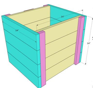
Now attach the other assembly you built in the first step the same way. Make sure touse wood glue in between the joints on the part and attach everything using 1.25" brad nails.
