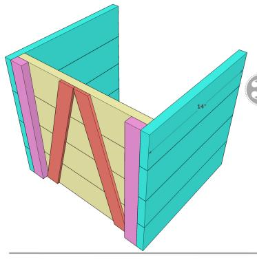
Add a line of wood glue on both ends of one of your side pieces and attach each side plank to it. They will line up side by side and flush with the sides you have already built. Attach the side boards using wood glue and 1.25" brad nails.
