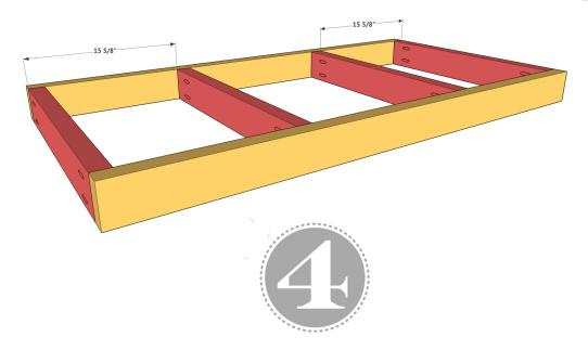
Cut the cross supports, drill 1 1/2" pocket holes in each end and attach them to the short frame pieces with 2 1/2" pocket hole screws and wood glue.
