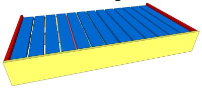
Finally, add a finish! Once the finish dries, attach to a wall, from the back frame piece into studs behind the wall.
