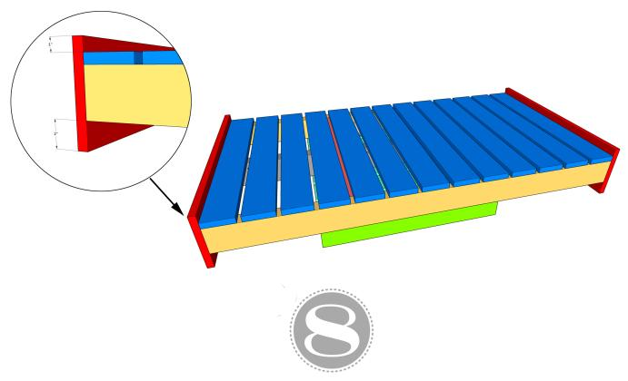
Cut the front of the bench to size. Attach it to the front of the frame with 1 1/4" brad nails and wood glue.
