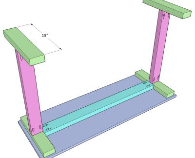
Attach the other two foot pieces next. These will attach to the legs using wood glue and 2.5" pocket hole screws through the 1.5" pocket holes. Make sure your pocket holes are facing the same direction on each leg because this will be the back of the desk that you won't see, so there will be no need to fill these pocket holes.
