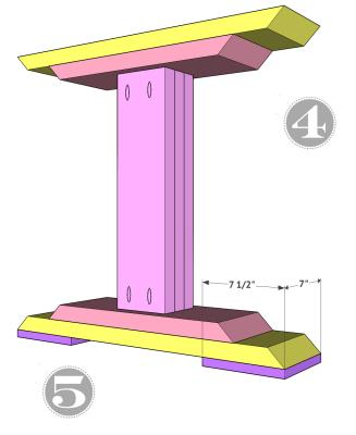
Now add the footpads. These are 1x8 boards that will sit the table off the ground a bit. It will give it stability and we love the look! Attach each footpad using wood glue and 1.5" Spax or wood screws.
