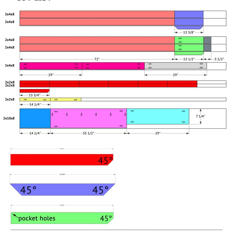
Note: I ripped the rounded edges off of every board making them 1/4" less wide. This is not a necessary step but if you choose not to, please adjust the measurements accordingly.
