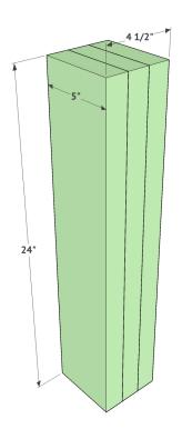
Now it's time to build the legs of this table. The center of these legs are also 2x6 boards that we ripped to 5". You will create two identical leg assemblies. Start by cutting the 3 leg base pieces and attach or laminate them using lots of wood glue and nails. You can use clamps to hold them tight in place until the glue dries. We like to let these set overnight, but you don't have to!
