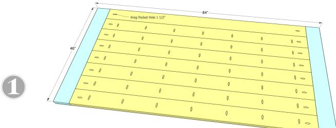
The first step to building this table is creating the table top. These are 2x6 boards that we ripped down to 5". We added 1.5" pocket hole screws down one long side of all but 1 of our plank boards, and also at the ends of each plank board. We attached the plank boards together first using 2.5" pocket hole screws. Once all plank boards are attached, line of the boards on each end and mark the exact measurement of the breadboards. Attach the breadboards using 2.5" pocket hole screws.
