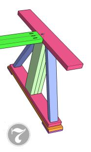
It's time to attach each leg assembly. Cut the runner to size and add 1.5" pocket holes to each end. Attach the runner to the center and flush with the top of each leg assembly. Use wood glue and 2.5" pocket hole screws to attach the runner.
