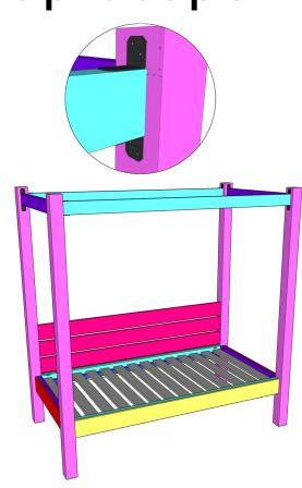
Cut the top slats to size and attach them to the top of the front and back frames with metal brackets.
