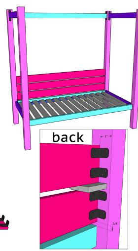
Cut the front and back apron pieces to size. Attach them to the frame pieces with 2 1/2" wood screws and wood glue. The top of the apron should be flush with the top of the frame.
