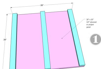
Attach the 1x2 boards to the project panel first using wood glue and 1.25" brad nails. Two of the boards will be flush on each side and the other board will be centered on the panel.
