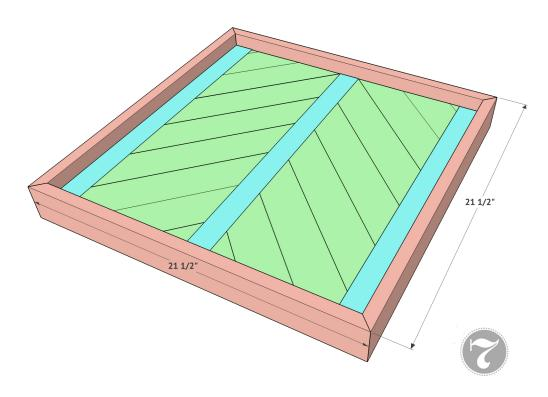
Measure and cut the rest of the trim boards to size and attach them to the outside of the panel using wood glue and brad nails. Now you are ready for legs! Be sure to check the website for a link to the legs we used. This would also make the cutest tray! Add a couple pulls to the sides and you are set! Have fun with it! Be sure to tag us and use hashtag #shanty2chic when you share your builds!
