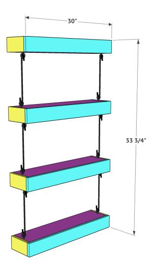
Slide the shelves over the cleats and secure with a wood screw on each end, from the top of the shelf, into the cleats. Check out the post on our site for details pics of how we added the hardware!
