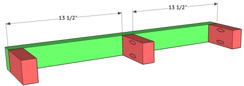
Cut the top and bottom plywood sheets to fit the length of the cleat and cut the side trim to the length of the cleat width. Attach the side trim pices to the top and bottom pieces with 1" brad nails and wood glue.
