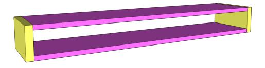
Cut the front trim piece to size and attach it to the shelf with 1" brad nails and wood glue.
