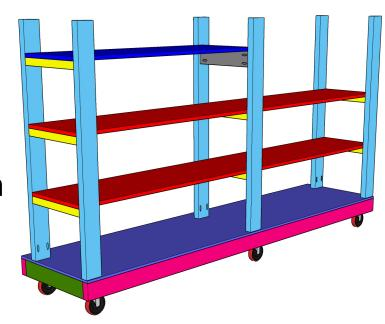
Cut the scrap, side panels to size and drill 3/4" pocket holes on the vertical sides.
