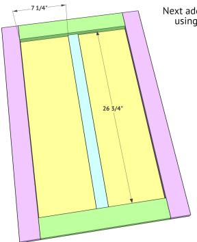
Next add the trim. Attach each piece using wood glue and 1/2" nails.
