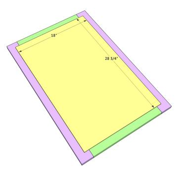
Next, attach the hardwood plywood panel to the back of each door. Attach using wood glue and 1/2" nails through the panel and into the back of the door frame.
