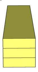
Cut the horizontal base planks to size. Center and attach one plank to the bottom end of the leg assembly with wood glue and 3" wood screws, from the bottom of the plank, into the leg assembly.
