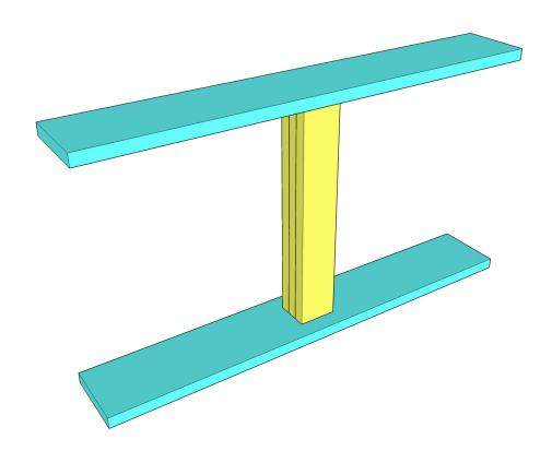
Cut the apron pieces to size. Drill 1 1/2" pocket holes into one edge of each piece. Attach the pieces together with 2 1/2" finish nails and wood glue. Note: make sure all of the pocket holes are facing the same way when assembling. Build two aprons.
