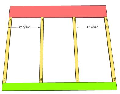
Cut the barn wood MDF to size and attach it to the frame with 3/4" staples and wood glue. If you don't have a stapler, you can use brad nails. Note: this door is covering a closet so I did not put a sheet of MDF on the back. If your door will be seen on the back side, you can attach a sheet of MDF on the back, the same way.
