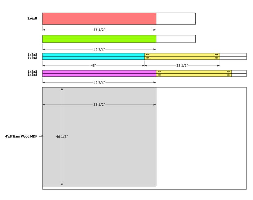
Cut the studs and top and bottom frame pieces to size. Drill 3/4" pocket holes at the ends of each stud. Attach the stud pieces to the top and bottom frame pieces with 1 1/4" pocket hole screws and wood glue.
