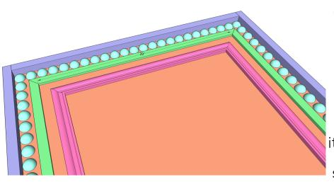
The final piece of trim to add is the small 3/4" trim. This will sit just to the outside of the half circles. If you can't find trim this size, you can easily create it by cutting a 1x4 or 1x6 board to 1/4" thick with a table saw. Attach each piece using wood glue and 3/4" brad nails.
