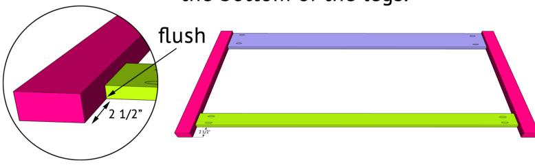
Cut the middle pieces to size and drill 3/4" pocket holes at both ends. Attach them to the top and bottom apron pieces with 1 1/4" pocket hole screws and wood glue.
