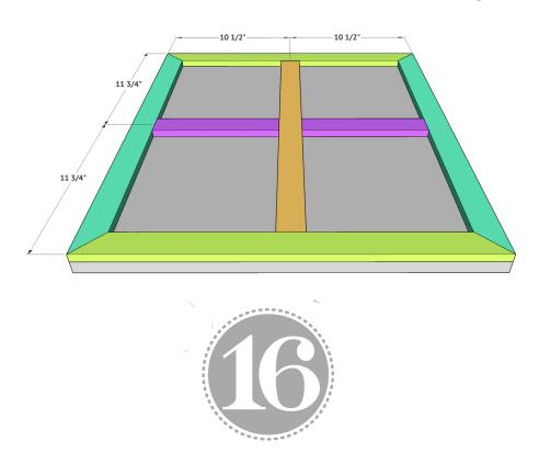
Cut the door side door trim pieces to size and attach them to the sides of the doors with 1 1/4" brad nails and wood glue. Measure and cut the top and bottom door trim pieces to size and attach them the same way.
