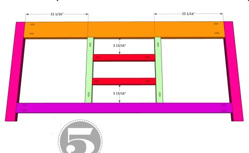
Attach the front face frame to the cabinet with 1 1/4" pocket hole screws and wood glue, from the cabinet bottom, side and middle panels and into the face frame. The cabinet bottom should be flush with the bottom apron. The side panels should be flush with
