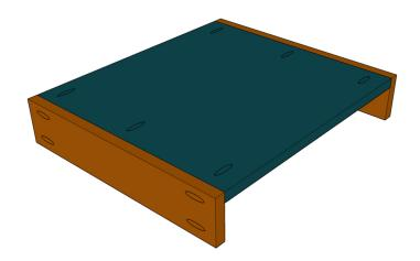
Cut the front and back pieces to size and attach them to the bottom and side pieces with 1 1/4" pocket hole screws and wood glue.
