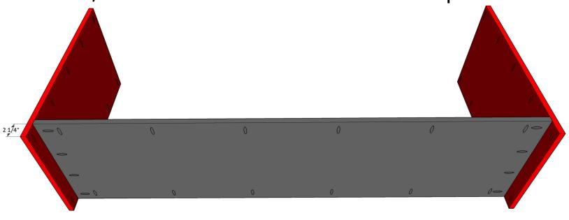
Cut the middle cabinet pieces to size and drill 3/4" pocket holes on the front and bottom edges. Attach them to the bottom of the cabinet with 1 1/4" pocket hole screws and wood glue.
