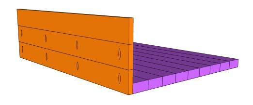
Cut the side planks to size. Measure and cut the vertical trim to fit. Attach the vertical trim to the ends of the planks with 1 1/4" brad nails and wood glue. Measure and cut the horizontal trim to size and attach it the same way. Build two assemblies.
