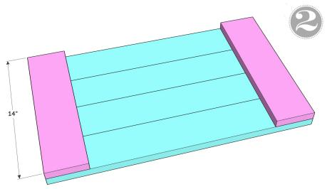
Cut the top pieces to match the measurement of all 4 boards placed side by side. If using 1x4 boards, that will be 14" long. If not, measure before you cut. Attach each end board flush with the ends of the longer boards using wood glue and 1.25" brad nails.
