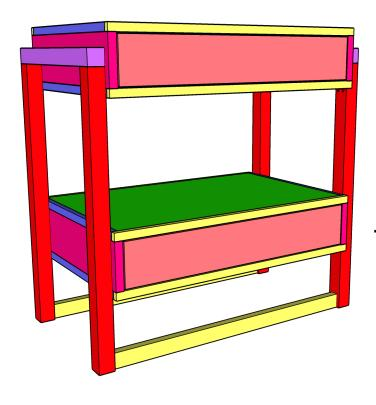
Cut the drawer faces to size and attach them to the drawers with 1 1/2" wood screws and wood glue, from inside the drawer and into the drawer face. Tip: with the drawer closed, place the drawer face where you want and hold it in place with a couple of brad nails.
