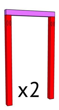
Cut the bottom rails to size and drill 3/4" pocket holes at both ends. Center the rails on the inside of the frames and attach them with 1 1/4" pocket hole screws and wood glue.
