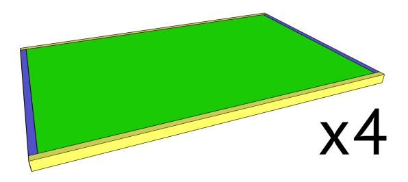
Cut the side shelf pieces to size, drill 3/4" pocket holes in one side of each board and attach them to the sides of the bottom shelf with 1 1/4" pocket hole screws and wood glue. Do this for both bottom shelves.
