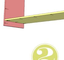
Assemble the face frame with pocket hole screws. The bottom board is centered with 3/4" overhang on both ends.
