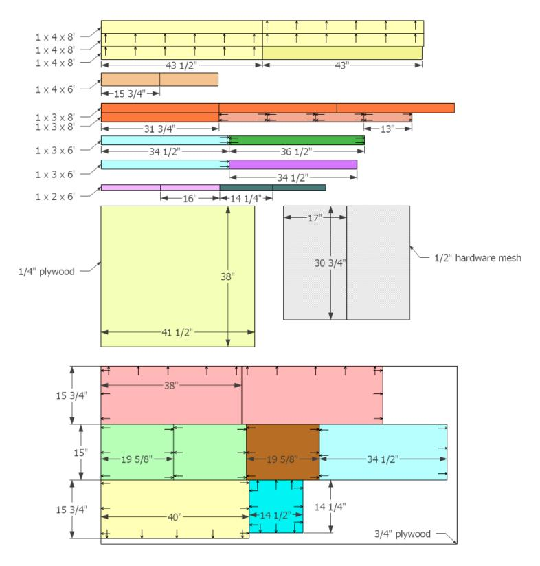
Drill pocket holes for 1-1/4" pocket hole screws as indicated by the arrows. Adjust all of your measurements as needed as they might be slightly different as you build.
