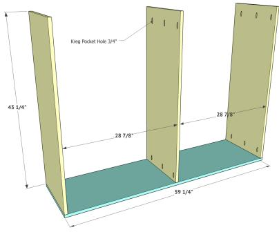
First, add 3/4" pocket holes to each end of all three vertical cabinet boards. Attach these boards to the base piece using 1.25" pocket hole screws and wood glue. Make sure the outside 2 boards are flush with the ends of the bottom board.
