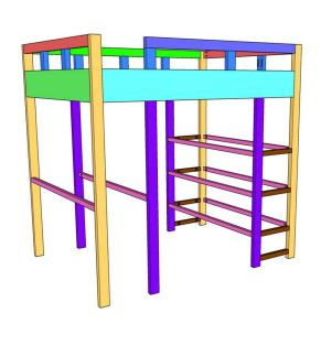
Cut the short desk pieces to size and drill 1 1/2" pocket holes in both ends. Attach them to the leg supports with 2 1/2" pocket hole screws and wood glue. The pocket holes on the bottom pieces will face in and the rest will face down.
