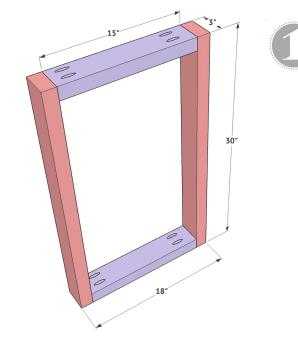
The first step of this project is preparing the 2 x 4 boards are used for the legs. Rip each 2 x 4 to 3" wide each give them a straight edge all around. Then, make shorter cuts. On the top and bottom leg pieces add 1.5" pocket holes on each side. You will build two identical leg assemblies for this desk. A Build a frame by attaching two of the short pieces to two of the long pieces using wood glue and 2.5" pocket hole screws.
