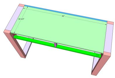
Attach this board flush with the top of your leg assemblies and also flush with your back apron using wood glue and 1.25" pocket hole screws through all of those pocket holes in into the desk.
