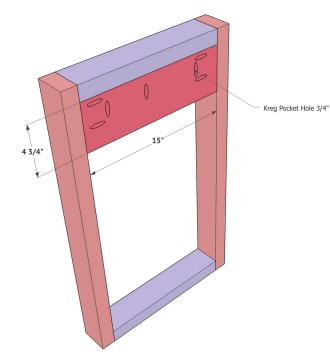
Once you have both leg assemblies built, attach the back apron board. This is a 1 x 6 board. Add 3/4" pocket holes to both short sides of the long apron board and also along one long side. When you attach this board, it will be flush with the top and back of each leg assembly. Attach it to the legs using wood glue in 1 1/4" pocket hole screws. You want your pocket holes on the apron board facing up or towards you.
