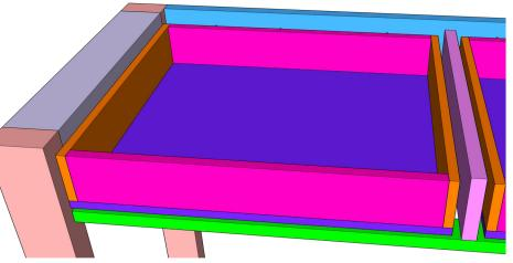
After you have attached the top of the desk, slide the drawer slides out and attach them to each of your drawers. There will be a half inch spacing on each side it will fit this drawer slide perfectly.
