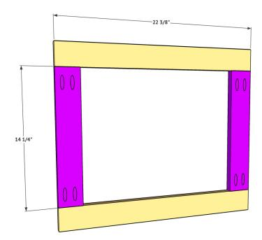
The face of the door is 1/4" plywood. Cut it to size and attach it to the back of the door frame using wood glue and 5/8" brad nails or staples. You can attach the door to the cabinet at this point, or add your finish first.
