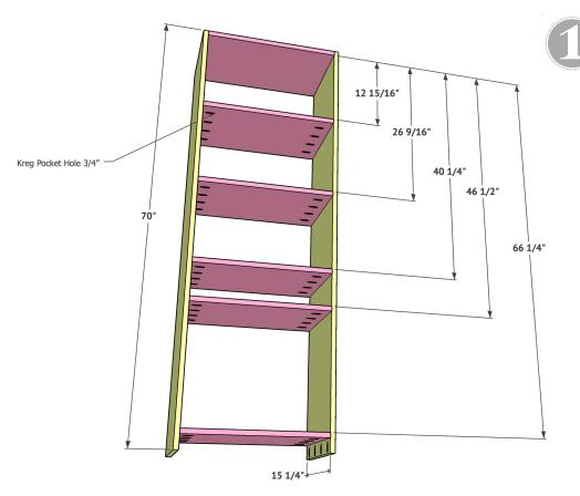
Build the body of the bookcase first. This is built with 3/4" thick Purebond Plywood. The front of each piece is edge banded to give a good finish, but that is optional. Add 3/4" pocket holes on each of the 6 shelf boards. Also, add 3/4" pocket holes on the inside bottom of both side pieces. Attach the shelves in place using wood glue and 1.25" pocket hole screws. Position pocket holes facing up on the top shelf board to hide them once the piece is finished.
