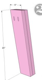
Next, create the leg pieces. These are 2 x 6 boards that I ripped down to 5" wide each. Cut to the correct length, and make sure each end is cut at a 10° angle. Add 1.5" pocket holes on one end of one board. The pocket holes will be on the inside and top of each leg, so be sure to glue each leg correctly. Glue these boards together and tightly clamp them until they are set and dry. Each leg will use two boards and you will have four legs total.
