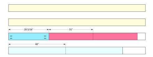
The first step to building this table is creating the table top. These are 2×6 boards that we ripped down to 5". We added 1.5" pocket hole screws down one long side of all but 1 of our plank boards, and also at the ends of each plank board., We attached the plank boards together first using 2.5" pocket hole screws. Onče all plank boards are attached, line of the boards on each end and mark the exact measurement of the breadboards. Attach the breadboards using 2.5" pocket hole screws.
