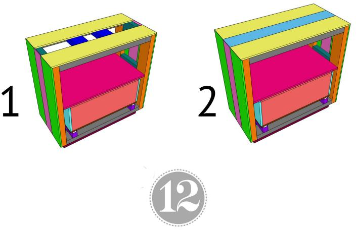
Cut the side, bottom trim pieces to size. Attach them to the sides of the pedestal with 1" pin nails and wood glue. Cut the front, pedestal trim piece to size and attach it the same way.
