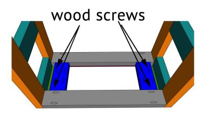
Cut the cleats to size, center them over the bottom cross supports and attach them with 2 1/2" wood screws from the top of the cleat into the supports.
