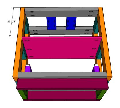
Cut the drawer sides, front and back pieces to size. Attach them together with 3/4" staples or brad nails and wood glue. Cut the drawer bottom to size and attach it to the drawer the same way. Attach the drawer to the drawer slides.
