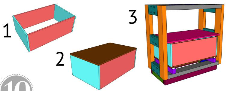
Cut the side trim pieces to size and attach them to the nightstand frame with 1" pin nails and wood glue. Start with the two outside pieces, then measure and cut for the middle piece. The bottom of the boards will be flush with the bottom of the nightstand frame, with the 45° cut on the top. Do this for both sides.
