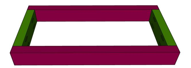
Attach the pedastal to the bottom of the nightstand, according to the image. Use 2 1/2" wood screws from the bottom of the inside of the nightstand and into the top of the pedestal.
