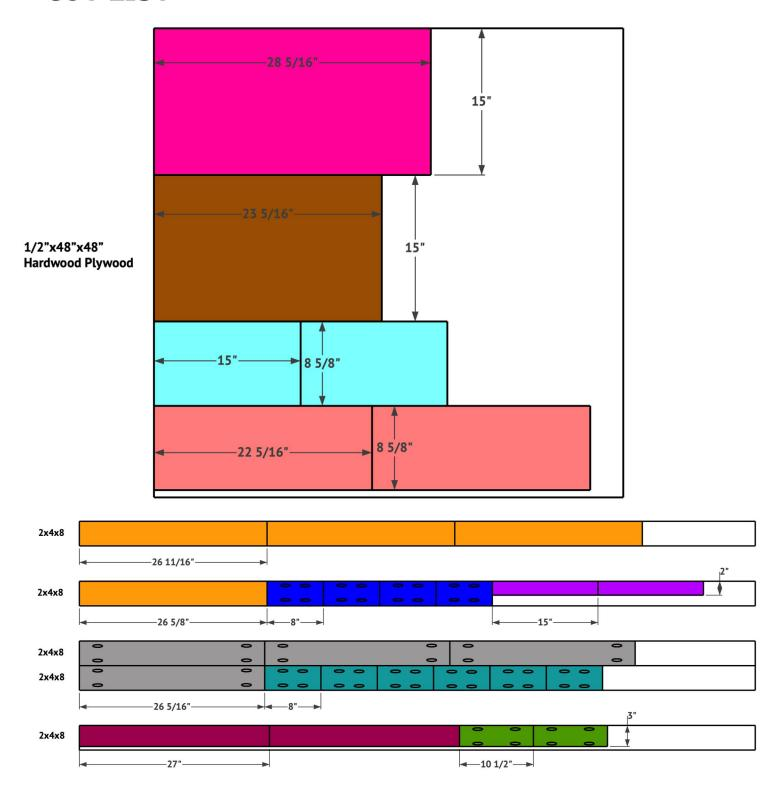
Cut the side frame pieces to size. Drill 1 1/2" pocket holes at both ends of the short cross pieces and attach them to the side pieces with 2 1/2" pocket hole screws and wood glue. Build 2 side frame assemblies.
