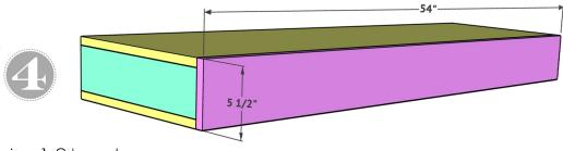
The front of the table is a 1x6 board. Cut the board to 54" and attach it to the piano hinge. Attach the magnetic closures to line up with the other end attached to the table.
