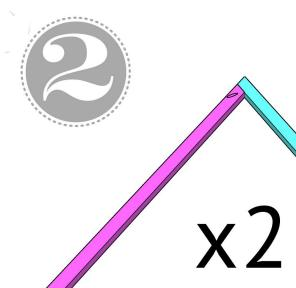
Attach the bottom frame piece to the side frame piece with 3/4" pocket hole screws and wood glue.
