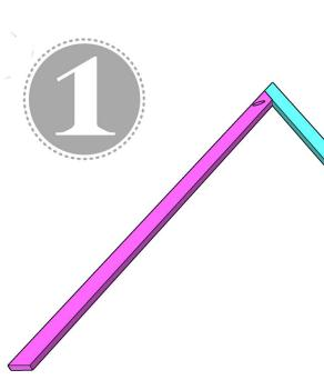
Cut the frame pieces to size and drill 3/4" pocket holes, according to the cut list. Attach the left and right frame pieces together with 1 1/4" pocket hole screws and wood glue.
