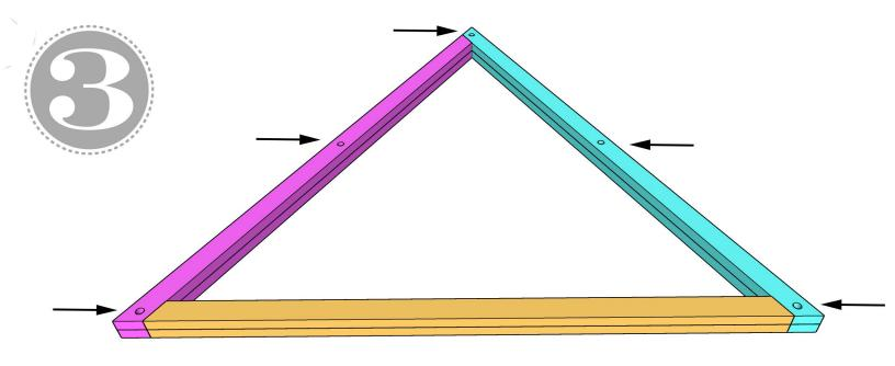
Stack the two frames on top of each other so that the pocket holes are facing down. With a 1/2" drill bit, drill a hole at every corner and the center of both side pieces. Make sure to use clamps to keep the frames in place while you drill.
