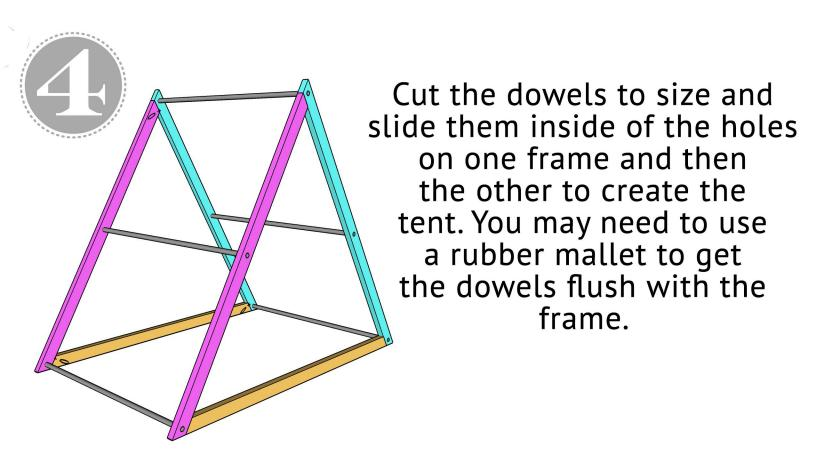
Once the dowels are attached, sand it down, fill your pocket holes and add a finish!
