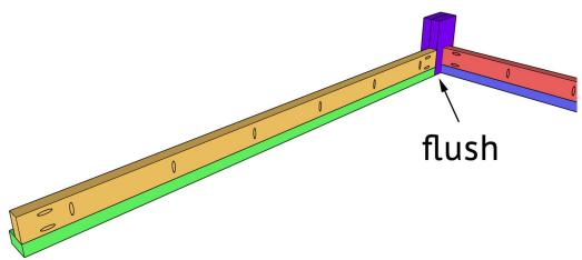
Attach the bed frame to the headboard with 2 1/2" pocket hole screws through the side rails and into the headboard legs. The inside of the rails and trim should be flush with the inside of the headboard legs.
