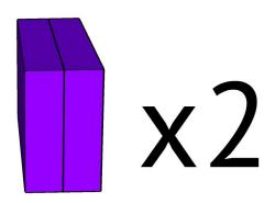
Cut the footboard trim to size and drill 1/2" pocket holes at both ends. Attach it to the feet with 2 1/2" pocket hole screws and wood glue. The front and top of the trim should be flush with the front and top of the feet.
