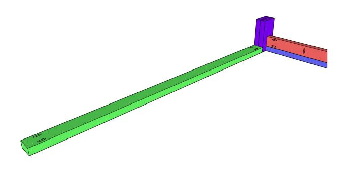
Cut the side rails to size and drill 1 1/2" pocket hole screws along one edge and both ends. Attach the rails to the trim and feet with 2 1/2" pocket hole screws and wood glue. The back of the rail should be flush with the back of the trim and inside of the feet.
