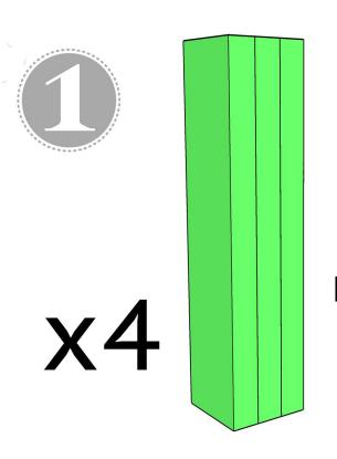
Cut the leg pieces to size. Stack 3 pieces together, with wood glue, and clamp for 24 hours. Build 4 leg assemblies.
