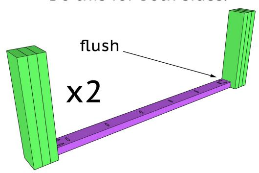
Cut the short apron pieces to size and drill 1 1/2" pocket holes on both ends. Attach them to the ends of both plank assemblies with 2 1/2" pocket hole screws and wood glue.
