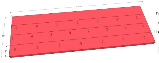
Build the top of the cabinet next. These are 2x6 boards that I ripped down to 5"wide each. Add 1.5" pocket holes down one side of 3 of the boards.
