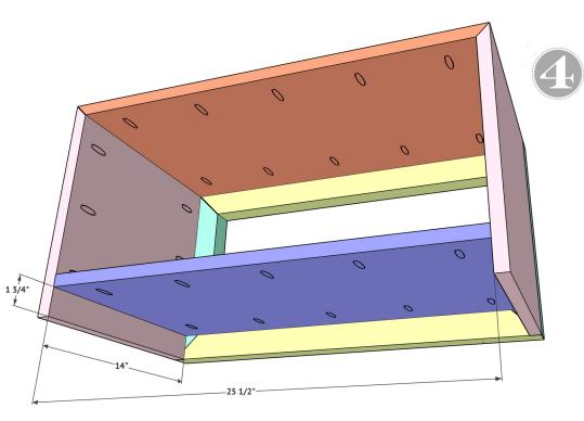
Next, attach the bottom board to the front frame. The bottom shelf board is made from one of the project panels. Add 3/4" pocket holes down both short and long ends of this board. Attach the board to the frame using wood glue and 1.25" pocket hole screws. The top of the bottom shelf will line up flush with the top of the bottom frame piece.
