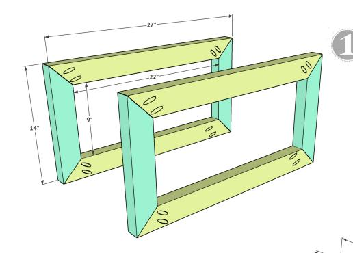
Create the frames first. These are made from 2x4 boards that I ripped to 2.5" wide each on the table saw. You will create 2 identical frames, one for the front and one for the back. Each piece will be cut at a 45° angle on each end. Add 1.5" pocket holes using your Kreq Jiq to the ends of each of the shorter frame pieces. You will do these also at a 45° angle. Attach the pieces to create 2 rectangle frames using wood glue and 2.5" pocket hole screws.
